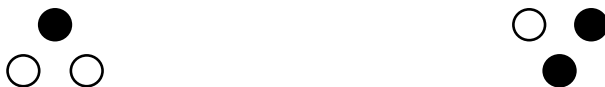
FIG 2. In this simple case, where k=3 , the set of black dots and the set of white dots have small Hausdorff distance but define two NN quantizers, say q_1 and q_2 , for which F_1(q_1, q_2) is large.
