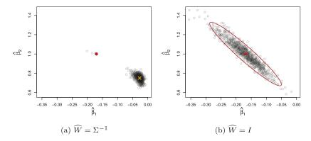
FIG 3. Parameter estimates using (a) standard WLS and (b) OLS when there is dependence between x and  $\sigma$ . We see that WLS is no longer consistent. The red point in each plot is the true parameter values. The orange  $\times$  in the left plot is the value to which standard WLS is converging (r.h.s. of Equation (3.9)). The red ellipse is the OLS sandwich asymptotic variance for the dependent case, Equation (3.2).
