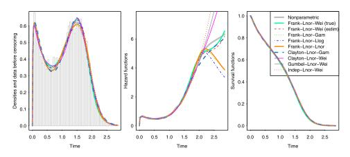
**Figure 5** Simulation 1. Comparison among the best copula model fitted. Density, hazard and survival functions for the polyhazard models of Table 1.
