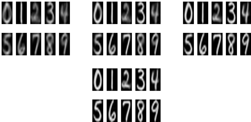
Figure 6. Evolution of the templates with the algorithm iterations. Top line – left: mean gray level images of the 20 training samples; middle: template at the 50th iteration; right: template at the 100th iteration. Bottom line: template at the 150th iteration. The improvement is visible, very fast for some very simple shapes, such as the digit ‘1’, and longer for very variable ones, such as the digit ‘2’. The higher geometric variability increases the fitting time of the algorithm.
