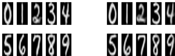
Figure 4. Estimated prototypes issued from left 10 images per class and right 20 images per class in the training set.
