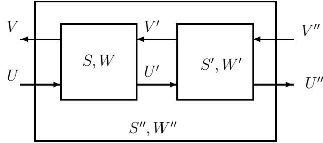
a scattering matrix  $S$  and the right one a scattering matrix  $S'$ . Using the notation of the figure, we have
