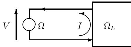
a voltage generator with internal impedance  $\Omega$  and which is loaded by an external load  $\Omega_L$ , then there will be a current
