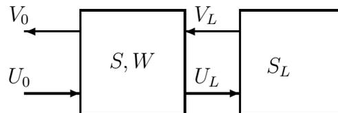
a 2-port which represents the left layer. Considering  $X = [U_0 \ V_L]^T$  as input and  $Y = [U_L \ V_0]^T$  as output for this 2-port, we have
