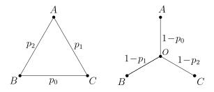
FIG. 3. The star-triangle transformation when  $\kappa_{\Delta}(\mathbf{p}) = 0$ .
