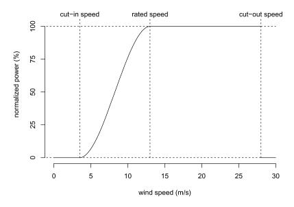
FIG. 1. Wind power curve. Wind turbine produces higher power as wind speed increases. A turbine starts power production at the cut-in speed, reaches its full operation at the rated speed, and stops producing power at and beyond the cut-out speed. Power outputs are normalized by the rated power.
