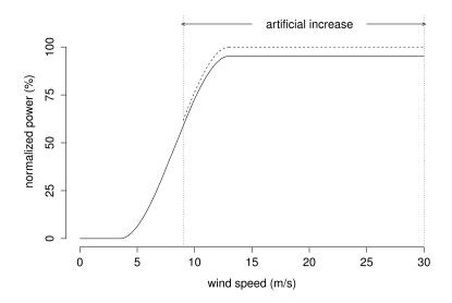
The modification in the mimicry test turbine data as if a pitch angle adjustment were ap-FIG. 3. plied. The power on the range of wind speed over 9 m/s is increased by 5%.
