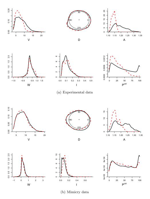
FIG. 4. Overlapped density functions of unmatched covariates and power output of control turbine; solid line = before upgrade (nontreated), dashed line = after upgrade (treated).
