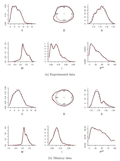
FIG. 5. Overlapped density functions of matched covariates as well as that of power output of control turbine; solid line = before upgrade (nontreated), dashed line = after upgrade (treated). Compare this figure to Figure 4 and notice the improvement in agreement between the pairs of density plots.
