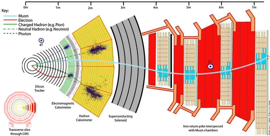
FIG. 3. Structure of the CMS experiment at the LHC [Barney (2004)]. The experiment uses layers of subdetectors to identify the particles created in proton-proton collisions and to estimate their properties. Copyright: CERN, for the benefit of the CMS Collaboration.
