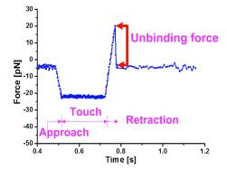
FIG. 2. One cycle of the unbinding force experiment.
