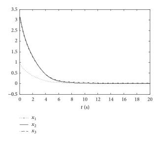
FIGURE 5: System responses under the control of the proposed FTC ((30a), (30b), (30c), (30d), and (30e)).
