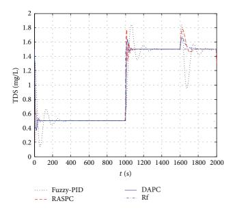
FIGURE 7: The response comparison in the presence of disturbance after the parameters change.
