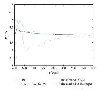
FIGURE 4: The response comparison in the presence of disturbance after the model changes.
