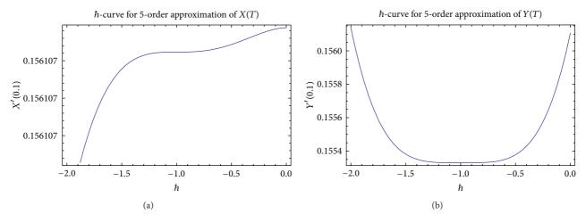
FIGURE 2: The  $\hbar$ -curves of X'(0.1) and Y'(0.1) obtained by the 5-order approximation of HAM.
