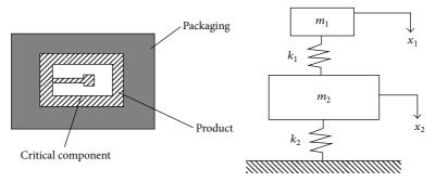
FIGURE 1: The model of packaging system with critical component  $(m_1 \ll m_2)$  and  $x_1 = x(t)$ ,  $x_2 = y(t)$ .
