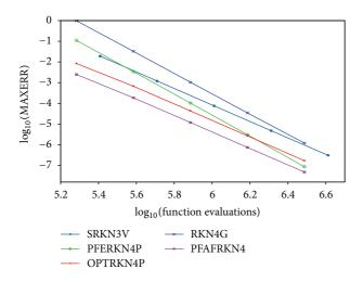
FIGURE 1: Efficiency curves for all methods for Problem 1 with e = 0 and  $h = 1/2^i$ , i = 3, ..., 7.
