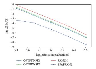
FIGURE 10: Efficiency curves for all methods for Problem 1 with e = 0.1 and  $h = 1/2^i$ , i = 3, ..., 7.
