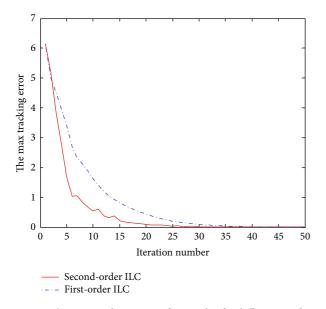
FIGURE 5: The max tracking error of Example 1 for different ILC laws.
