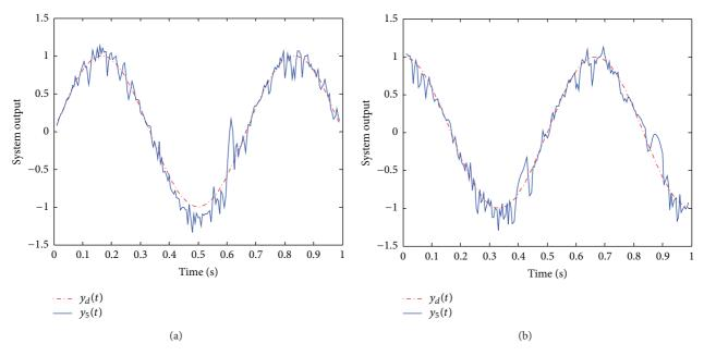
FIGURE 7: System output trajectory at 5th iteration for Example 2: (a)  $y_{1,k}(t)$ , (b)  $y_{2,k}(t)$ .
