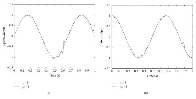
FIGURE 8: System output trajectory at 10th iteration for Example 2: (a)  $y_{1,k}(t)$ , (b)  $y_{2,k}(t)$ .
