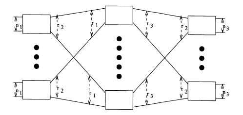
FIG. 3. Three-stage Clos network.
