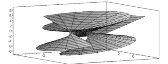
Fig. 3.1. A rotational ruled surface of the first kind with a = 2.
