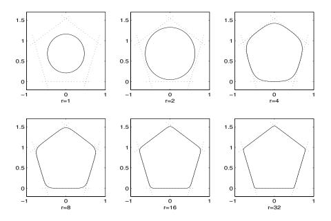
Figure 2: Plots of the pseudo-characteristic function  $F_r(x, y)$  for different values of r for the pentagon of section 3. The boundary of  $F_r$  "balloons out" to fill the polygon P; we note that it is possible to construct a modified function  $F'_r(x, y) = \eta F_r(x, y)$  which "shrink-wraps" onto P by choosing  $\eta = 1/\max_j (F_1(v_j))$  where the  $v_j$  are the polyhedron vertices.
