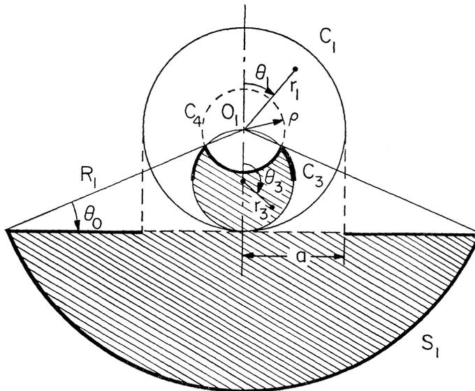
FIG. 1 The geometry of the Kelvin inversion.
