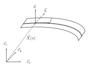
**Figure 1.** The connection between the Frenet frame  $\{\vec{t}, \vec{b}, \vec{n}\}$  on the central curve of the insulator layer and Cartesian coordinates. The *s* coordinate parameterizes the central curve.
