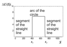
**Figure 3.** The potential barrier formed in the region of constant curvature (i.e., K(s) = 1/R for  $s \in [s_1, s_2]$ ). This picture is valid whenever  $0 < s_1 < s_2 < l$ . The parameters in the plot are the following a = 20,  $R = 200, b = 100, l = 1000, s_2 = 700, s_1 = 400$ .
