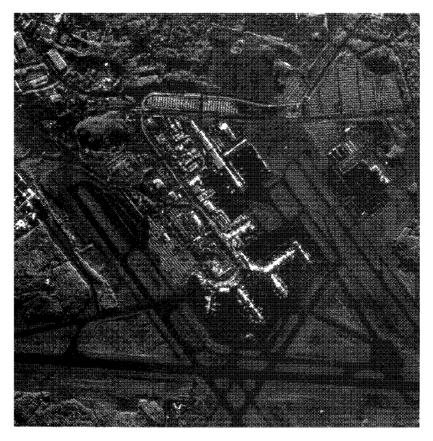
**Figure 6.** High resolution microwave radar image of the Baltimore–Washington International (BWI) Airport obtained with a microwave SAR modality designed for an unmanned aerial vehicle. The holographic signal processing makes the resolution independent of the sensor's altitude
