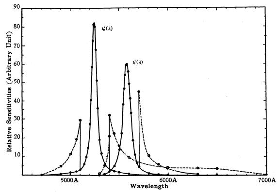
Fig. 3.1 Relative Sensitivities of the Photometer using the GreenLin e or the Control Filter,  $t_1(\lambda)$ ,  $t_2(\lambda)$  in Arbitrary Unit.
