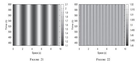
In FIGURE 21, we set (p,q) = (1.5, 1.7),  $(d_1, d_2, d_3) = (0.02, 0.96, 0.02)$ , and in FIGURE 22, we set (p,q) = (1.5, 2.7),  $(d_1, d_2, d_3) = (0.004, 0.166, 0.83)$ . Plotted in these figures are the numerical solutions u(x, t) of (3.1), solved by semi-implicit schemes under the homogeneous Neumann boundary conditions.
