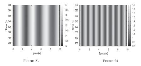
Parameter values are (p,q) = (1.5, 3.5),  $(d_1, d_2, d_3) = (0.1, 0.65, 0.25)$  in FIGURE 23, and (p,q) = (1.2, 3.5),  $(d_1, d_2, d_3) = (0.02, 0.15, 0.83)$  in FIGURE 24. The numerical solution u(x, t) of (3.1) is plotted.
