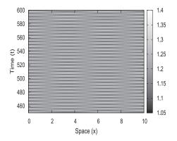
FIGURE 25. In FIGURE 25, we set  $(p,q) = (1.2, 3.5), (d_1, d_2, d_3) = (0.02, 0.09, 0.89)$ , and the numerical solution u(x, t) of (3.1), solved by semi-implicit schemes under the homogeneous Neumann boundary conditions, is plotted.
