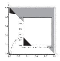
FIGURE 20. We set (p,q) = (1.2, 3.5) in FIGURE 20. The pair  $(d_1, d_3)$  is in the white area if  $p_1(\mu)p_2(\mu) - p_3(\mu) = (d_1 - d_1^2 + d_3 - 2d_1d_3 + d_1^2d_3 - d_3^2 + d_1d_3^2)\mu^3 + (-0.5 + 2.88d_1 + 0.66d_1^2 + 2.88d_3 - 2.88d_1d_3 - 2.44d_3^2)\mu^2 + (3.85 - 1.1764d_1 - 4.9664d_3)\mu + 0.2708 > 0$  for all  $\mu > 0$ , and it is in the black area if  $p_1(\mu)p_2(\mu) - p_3(\mu) < 0$  for some  $\mu > 0$ . W-instability occurs on the boundary between these areas.
