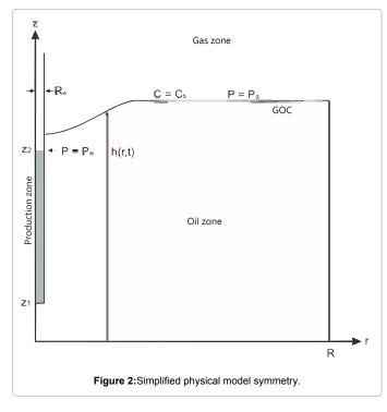
The first one describes the nitrogen dispersion far away from the wells; the second one describes the nitrogen dispersion in the neighborhood of a producer well. Both cases are formulated in a homogeneous porous media and for simplicity it is considered that the oil saturation in the oil zone,  $S_{oi}$ , is constant and that in the gas zone the oil concentration,  $S_{oi}$ , is also constant.
