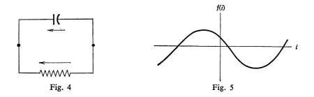
Here i, f(i) are the current and voltage in the resistor where we assume that f has the qualitative properties indicated in Fig. 5. Let i be a parameterization of  $\Sigma$  so that
