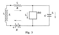
Here L, the resistance R in branch 2, and C are all linear. E is the constant voltage source and can be thought of as a resistance with characteristic  $(i_1, v_1) = (i_1, E)$  and the resistance in branch 3 is voltage controlled with characteristic defined by the function f on **R**.
