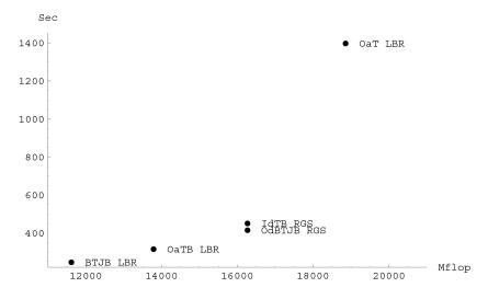
Figure 11. A plot of the more interesting results from Figures 8 and 9 with the number of Mflops on the x-axis and the running time in seconds on the y-axis. Each point is labeled with the permutation applied and the solving method used. The best performance of a method, which permutes the node in separating them into dangling and nondangling without applying any BFS visit, is plotted with the best block and scalar methods that use one or two BFS visits.
