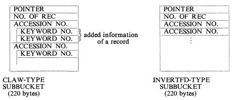
Figure 7.5 Structure of buckets of GHUBFS<sub>2</sub>
