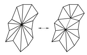
**FIGURE 7**. Expansion (respectively contraction) of an edge.
