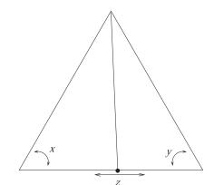
**FIGURE 1**. By splitting a triangle from a vertex, we are led to a system with three degrees of freedom: x, y, and z in the figure.
