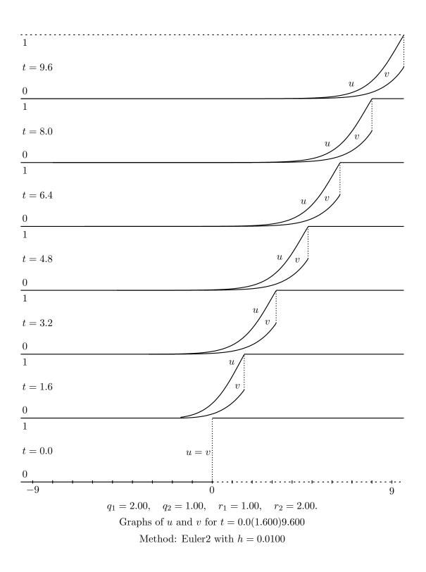
Figure 4: Numerical solution calculated using modified Euler method along the characteristics
