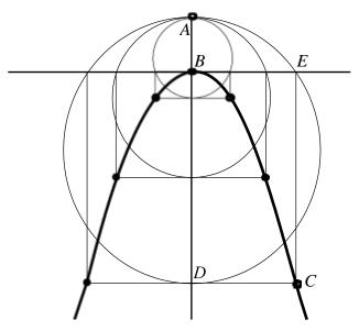
Figure 19.6 Construction of parabola
