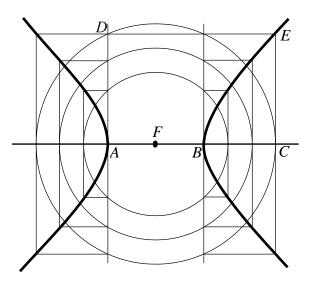
Figure 19.8 Construction of hyperbola
