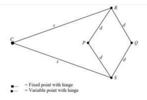
Figure 16.7 A linkage for constructing an inversion
