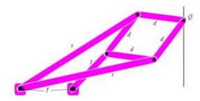
Figure 16.8 Linkage for drawing a straight line
