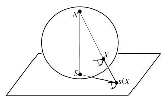
Figure 14.3 Stereographic projection is angle-preserving
