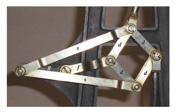
Figure 1.5 Peaucellier/Lipkin linkage for drawing a straight line
