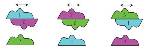
Figure 1.2 Grinding flat mirrors
