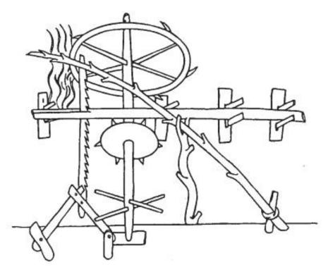
Figure 1.3 Up-and-down sawmill of the 13<sup>th</sup> century
