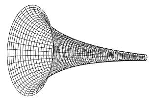
FIGURE 4. A portion of a pseudosphere, which extends to infinity at the thin end. A pseudosphere is a surface of revolution of Gaussian curvature -1. The generating curve is a tractrix, which is characterized by the property that its tangent lines meet the x-axis a unit distance from the point of tangency.
