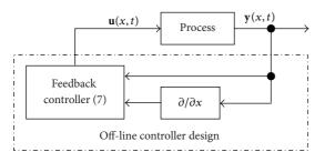
FIGURE 1: The structure of distributed P-sD state-feedback controller.
