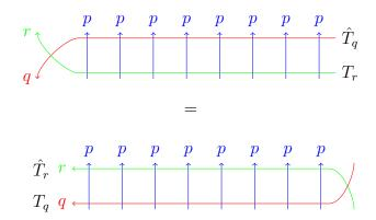
FIGURE 6. Commuting Transfer Matrices: Shown here is the result of repeated application of the Star-Triangle Equation. Applying an additional qr weight to the right before closing the q and r rapidity lines, we can apply the inversion relation and prove that the transfer matrices commute.
