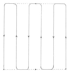
Figure 1. Typical flight path during an aeromagnetic survey.
