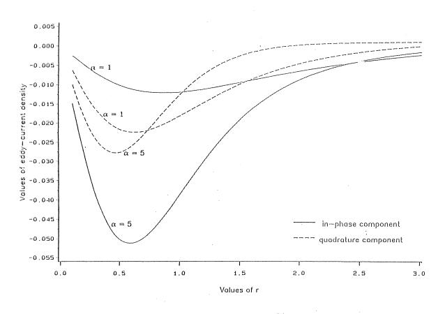
Figure 1. Zeroth order current density,  $j_{\theta}^{(0)}$ , as a function of r for  $\alpha = 1$  and 5.
