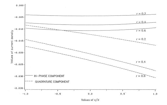
Figure 2. Current density variation across the thickness of the sheet at three different values of r.  $\alpha = 1$ ,  $\lambda = 1$  and  $\delta = 0.1$ .
