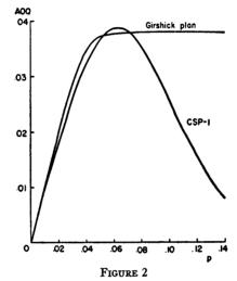
Comparison of AOQ curves for Girshick sequential (N = 400, m = 16, f = .05) and CSP-1 (i = 38, f = .05).
