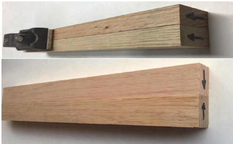
Figure 1.1 Cabinet maker's method for checking straightness
