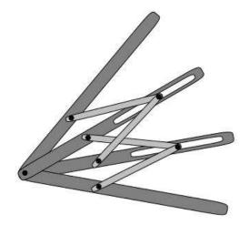
Figure 15.11 Mechanism to trisect an angle
