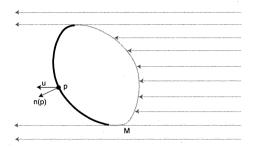
Fig. 1. The shadow cast on a surface M, when illuminated by light rays parallel to u corresponds to points p in M where the inner product between u and the unit normal n(p) is positive.
