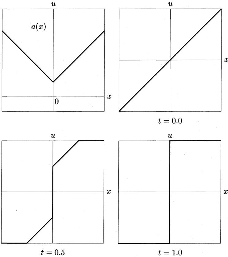
Fig. 8. Simulation of Example 4.1 with  $a(x) = 0.2 + |x|$ ,  $b(x) \equiv 1$  and  $u_0(x) = x$ . Discontinuity appears instantaneously and the solution reaches to the final state in a finite time.
