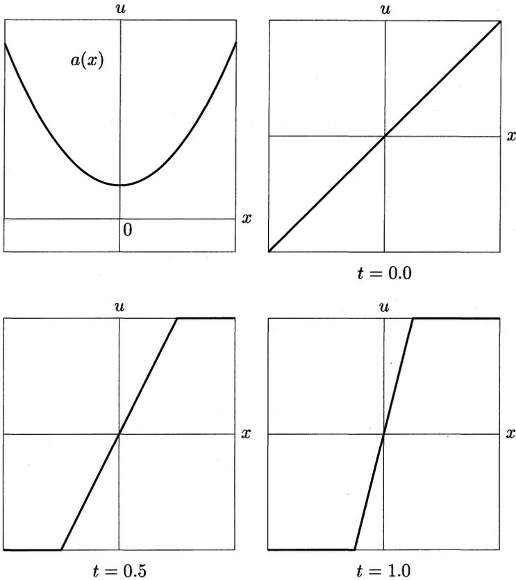
Fig. 9. Simulation of Example 4.2 with  $a(x) = 0.2 + x^2$ ,  $b(x) \equiv 1$  and  $u_0(x) = x$ . Discontinuity never appears and the solution converges to the final state while it doesn't reach the final state in a finite time.
