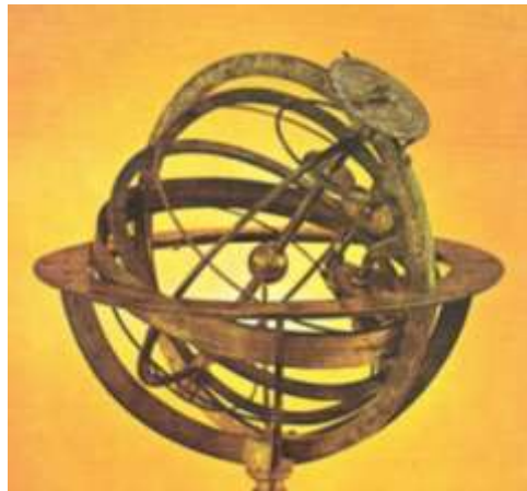
Figure 2.1 Armillary sphere (1687) showing (from inside out): earth, celestial sphere, ecliptic, and the horizon
