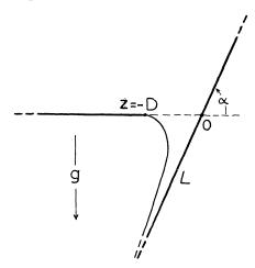
supported by a semi-infinite horizontal plane, and is bounded on the right by an infinite plane inclined at an angle  $\alpha$  with the horizontal. The flow is downward through an open slot in the horizontal plane into a jet with a free boundary extending to infinity. This family includes the case of the symmetric jet from a slot, obtained when  $\alpha = \pi/2$  by reflecting the flow across the vertical boundary.
