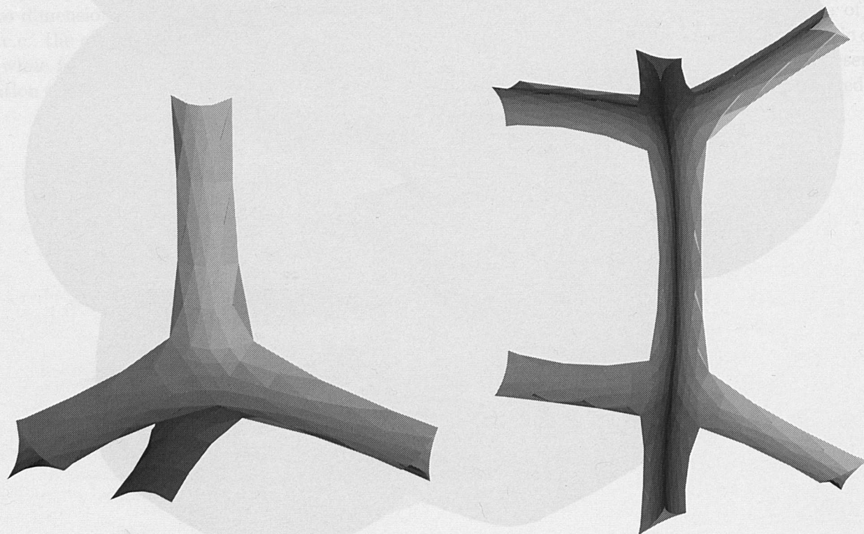
FIGURE 8. Left: A single vertex from the Plateau border network. The four edges, approximately triangular in cross section, meet at the tetrahedral angle. Right: A more extended sample of the Plateau border network, showing two vertices.
