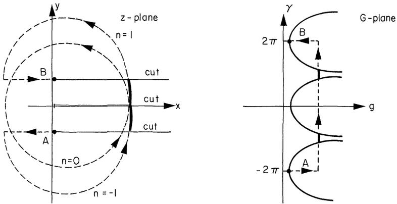
**Fig. 4.** Mapping of a rectangle in the  $G$  plane onto the  $z$  plane. The broken parts within the cigars map onto (almost) circular loops in different  $z$  sheets, from where they emerge at the corresponding cuts to continue (fat full curves) in the principal sheet to the next cut, where they dive to another sheet for another loop
