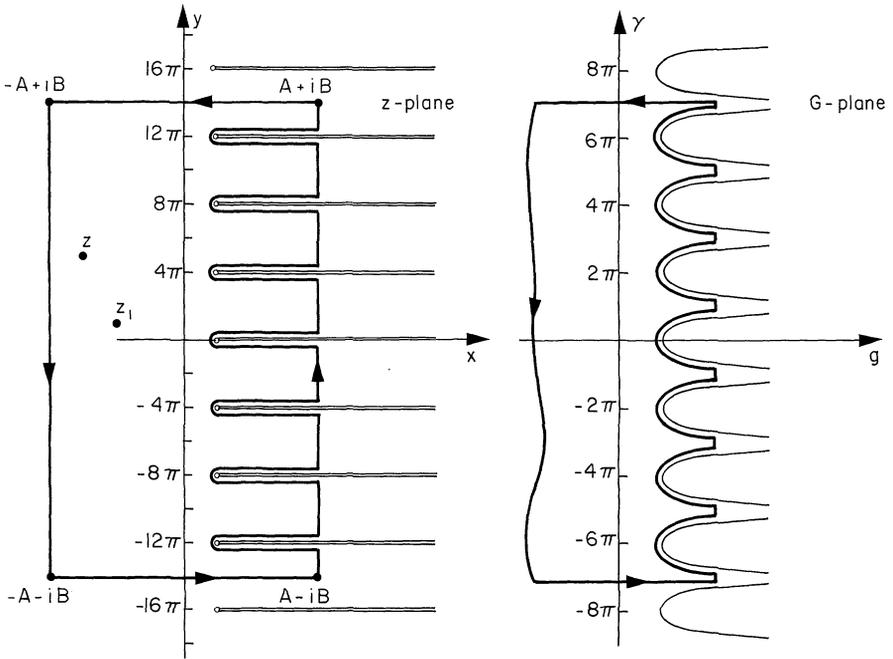
**Fig. 6.** The integration path for Eqs. (4.1) and (4.2), shown in the  $G$  and  $z$  planes (principal  $z$  sheet). This path is pushed to  $\infty$  in all directions in the order first  $B \rightarrow \infty$ , then  $A \rightarrow \infty$ . Apart from the cuts, the vertical boundary lines give a finite contribution
