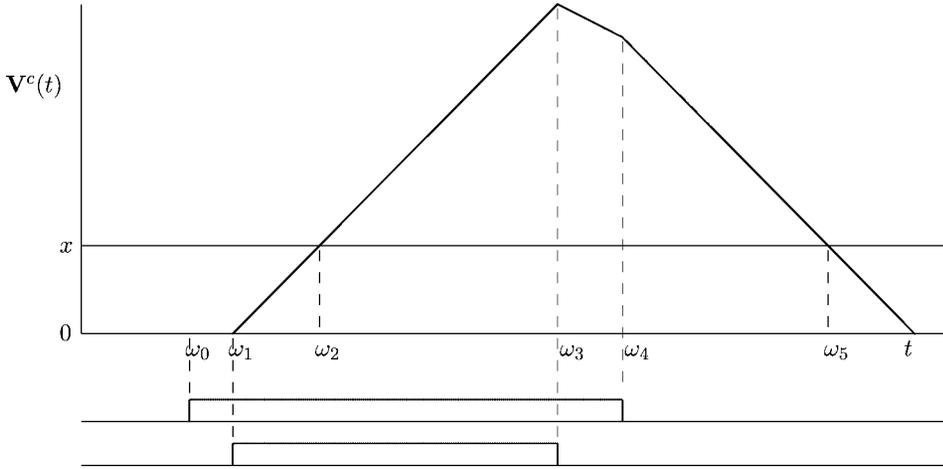
FIG. 1. Typical overflow scenario for two On-Off flows.
