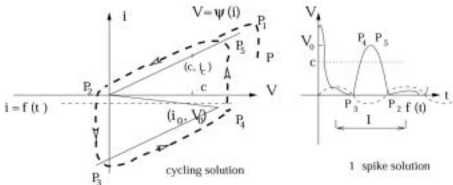
Fig. 3. Spike solution and spike solution when  $0 > f(t) > i_0$
