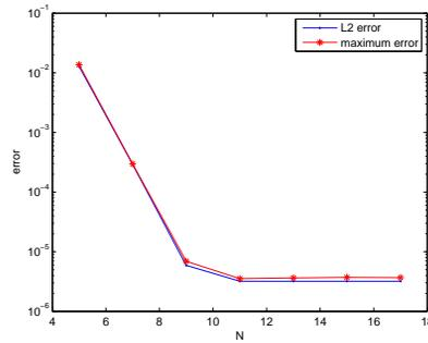
Figure 5.2: Errors as a function of the polynomial degree  $N$  for  $\alpha = 0.8$ .
