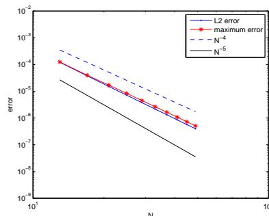
Figure 5.3: Errors as a function of the polynomial degree  $N$  for  $\alpha = 0.1$ .
